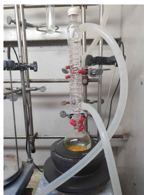
Figure 5. Heating under reflux
