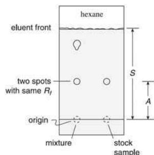
**Figure 2.** A chromatogram showing measurement for  $R_f$  calculations
