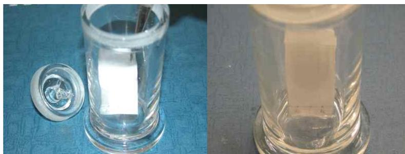
Examine the developed TLC plate under a UV light (254 nm). Use a pencil to circle any visualized spots. A reagent such as anisaldehyde or phosphomolybdic acid solution is sprayed on the plate. This reagent formed a colored product with the compound of interest.
