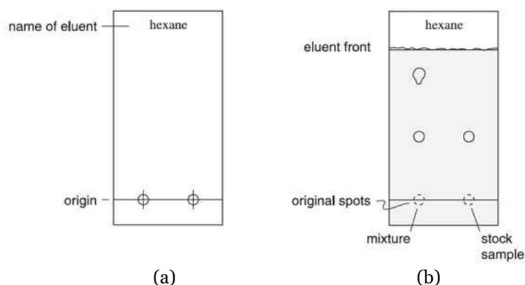
During the TLC process, the solid stationary phase, called the **adsorbent**, adsorbs the mixture compounds. As the mobile phase, called the **eluent**, travels up over the adsorbent the compounds within the mixture move at different rates. A reversible and continuous competitive attraction between the eluent and the adsorbent for the mixture compounds causes this rate difference.
